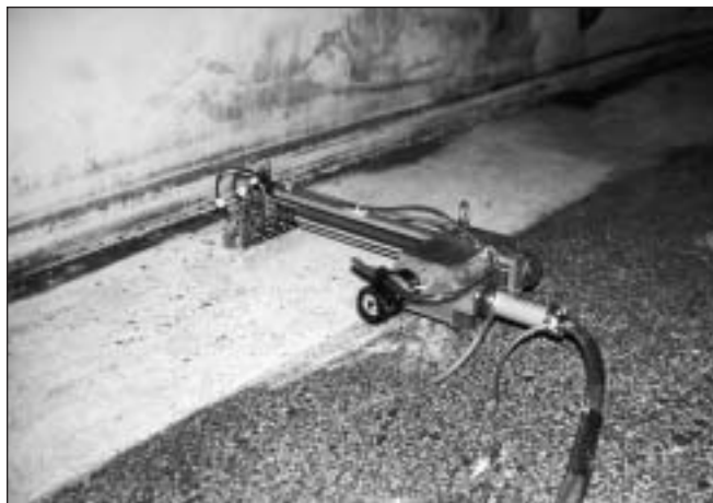
Here's an example of an automated ultrasonic bottom-scanning device (Fig. 3).
